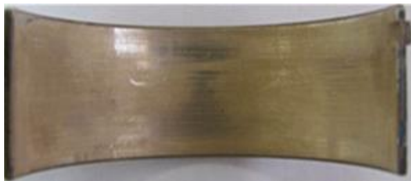
Fig.4 SV Bearing after One Season of Racing
